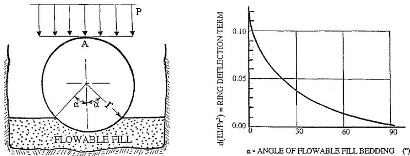
**Figure 5a, b: Flowable Fill Bedding, Ring Deflection-Bedding Angle Relationship (ASCE 2009)**
