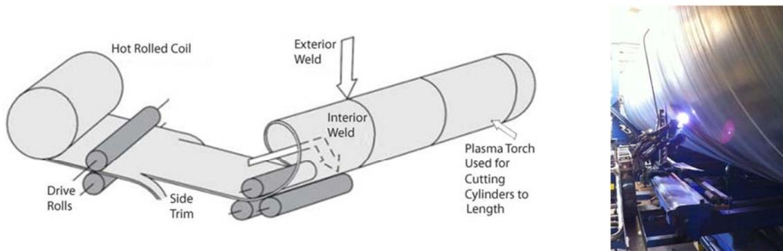
**Figure 2a, b: Spiral-Welded Steel Pipe (AWWA 2004), Plasma Torch for Cutting Cylinders to Appropriate Lengths**
