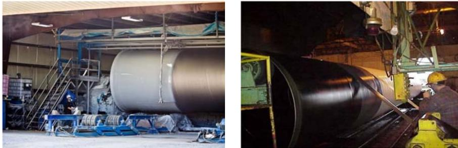
**Figures 2a, b: Polyurethane Coating, Tape Coating**
