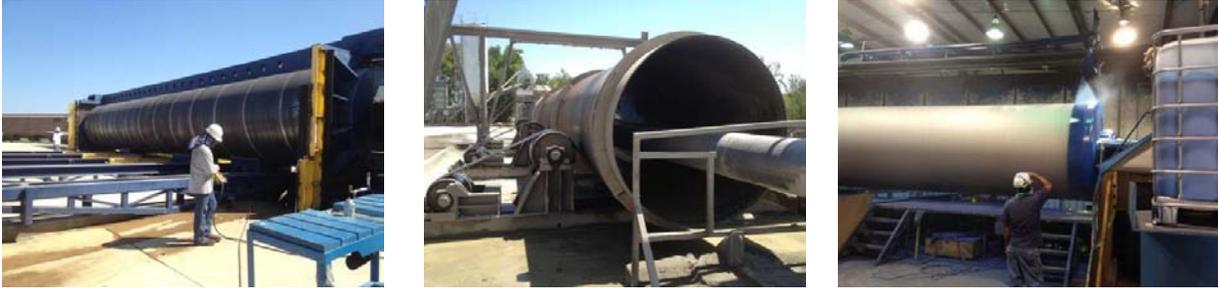
Figures 6a, b, c: Hydrostatic Testing, Cement Mortar Lining, Polyurethane Coating
