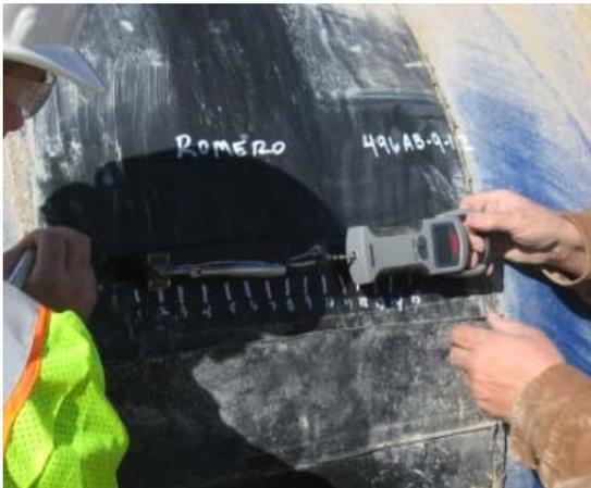
Figure 3 – Horizontal peel test
