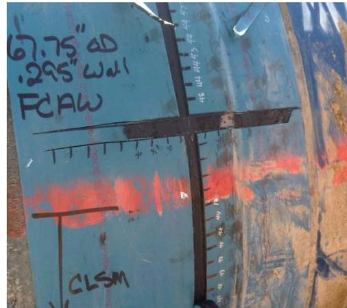
Figure 4 – Sleeve after completed test
