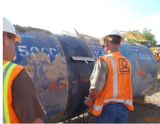
**Figure 2 – Holiday testing of sleeve after removal from trench**
