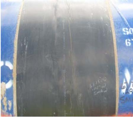
**Figure 1 – Heat shrink sleeve after removal from trench**
