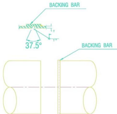
**Figure 3** Beveled Joint in Contract Drawings
