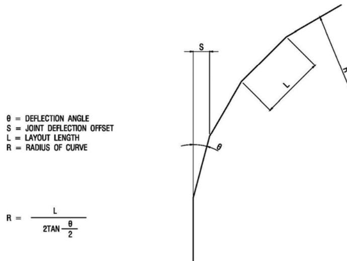
**Figure 2** Route Geometry Calculation to Determine Joint Deflection
