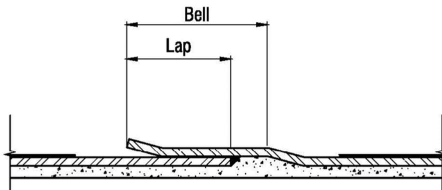
**Figure 5** Hybrid Lap-Welded Joint for Steel Water Pipe
