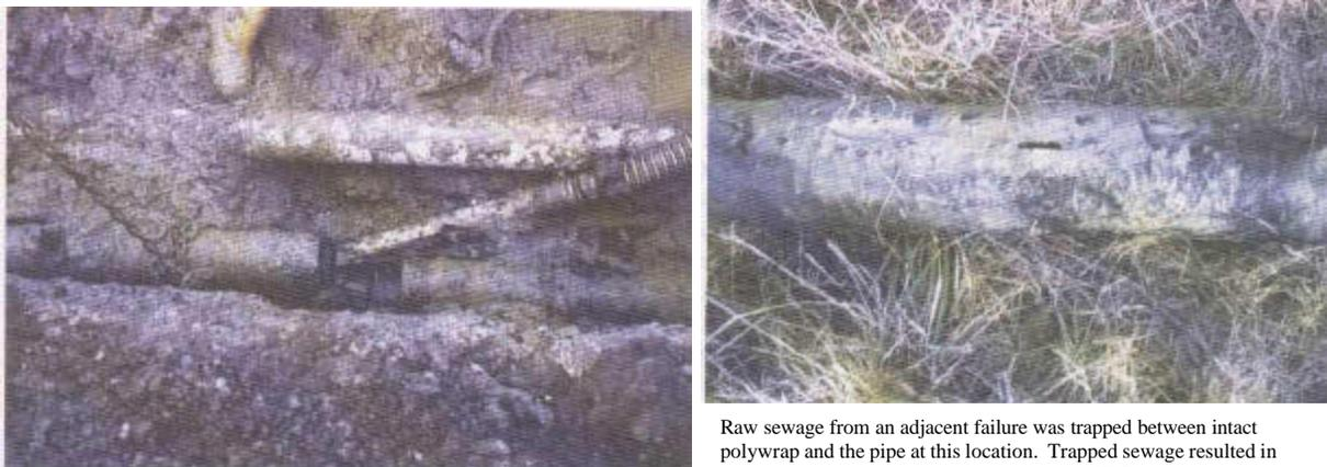
A section of failed polywrapped pipe being removed. Failure occurred from external corrosion at breaks in the wrap.
