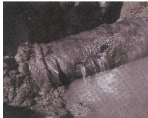
5-year old ductile-iron pipe in polyethylene encasement
