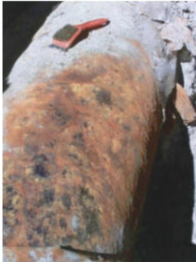
Less than 25-year old ductile-iron pipe in Northern California.
