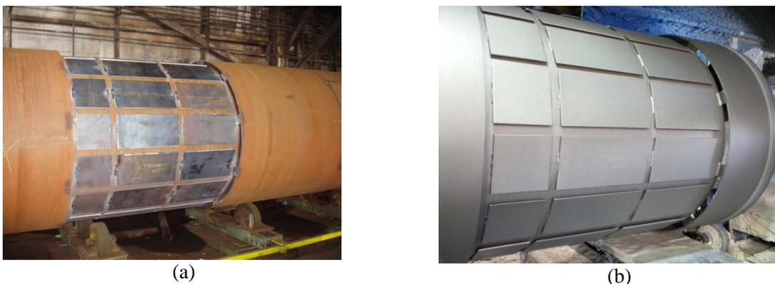
Figure 1. Pipe with smaller diameter section to accommodate flat panels for the cleaning and coating processes (a) prior to blasting, (b) after blasting.
