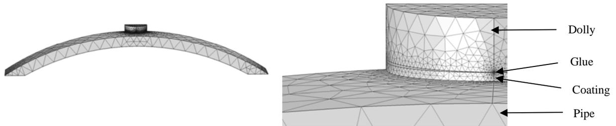
*Figure 2. Overall and detailed view of the mesh used in the finite element computer simulation of the pull-off test on a pipe. The coating beyond the scoring around the dolly is not included since it is separated from the coating under stress.*
