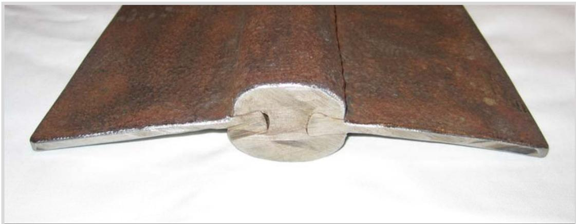
**Figure 2 : Lock-Bar Pipe Joint**
