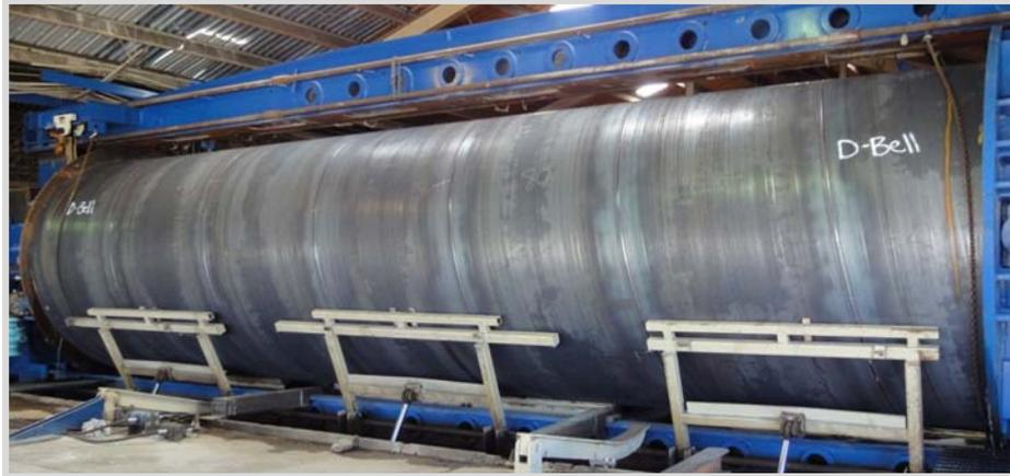
**Figure 3 : Spiral Welded Steel Pipe, 126” Diameter (During Hydrotest)**
