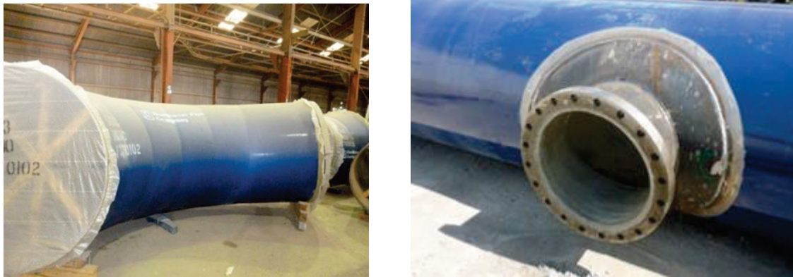
Figure 1. (a) Mitered steel pipe bend for large-diameter pipeline; (b) reinforced 90-deg steel pipe outlet (photos by Spyros Karamanos).
