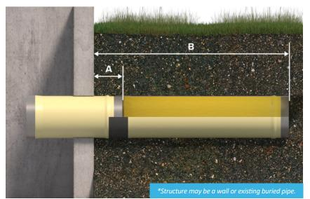
Then, refer to this figure to determine the location of the required InfraShield<sup>®</sup> projection(s).
