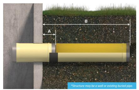
First, determine whether one or two InfraShield<sup>®</sup> projections are required in the pipeline design. Use the table to match the to the amount of expected settlement with the pipe diameter.
