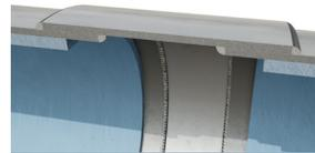
Features a two-piece roll formed strap that joins pipe with two longitudinal welds in addition to a circumferential fillet weld.
