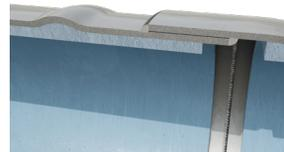
Builds on the bell-and-spigot lap weld joint by adding a small projection in the pipe wall that protects joints during settlement and geohazards.
