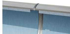
Single-weld circumferential joint that allows up to 5° deflection with a miter cut on one end or 10° deflection joining two mitered ends.
