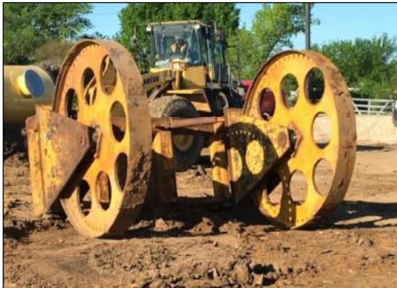
Figure 7: Wheel Compactor for CSS Embedment
