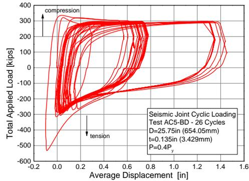
**Figure 12. Load-displacement curve of axially-loaded AC5-BD-SR specimen; positive values of axial force correspond to compressive loading.**
