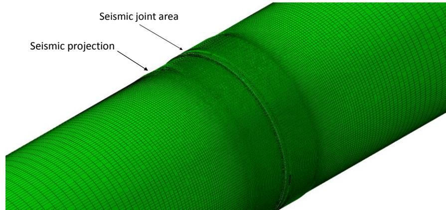
**Figure 4. Finite element mesh of the numerical model for the ATLAS SR-joint.**
