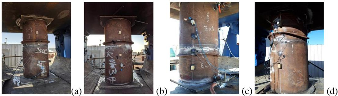
Figure 9. Local buckle configuration in axial compression experiments; (a) AC1-AD-SR, (b) AC2-ASO-SR, (c) AC3-BD-SR, (d) AC4-BSO-SR; all specimens buckled at the spigot side, where the artificial “seismic projection” was imposed.
