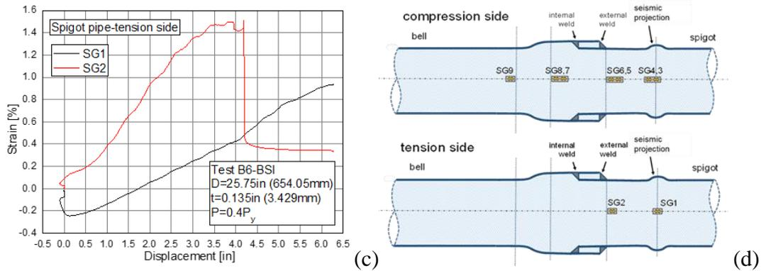
Figure 10. Strains with respect to applied displacements for bending test B6-BSI-SR.
