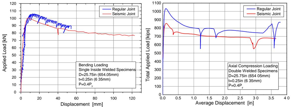
Figure 7. Load-displacement curve under four-point bending of the seismic joint with respect to the regular joint (Keil *et al.* 2018); (a) specimen B3-ASI-SR; (b) specimen AC1-AD-SR.
