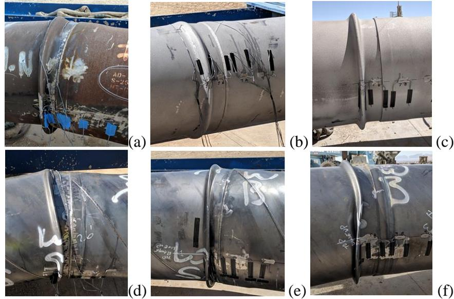
Figure 8. Local buckle configuration in bending experiments; (a) B1-AD-SR, (b) B2-ASO-SR, (c) B3-ASI-SR, (d) B4-BD-SR, (e) B5-BSO-SR, (f) B6-BSI-SR; all specimens buckled at the side of the spigot, where the artificial “seismic projection” was imposed.
