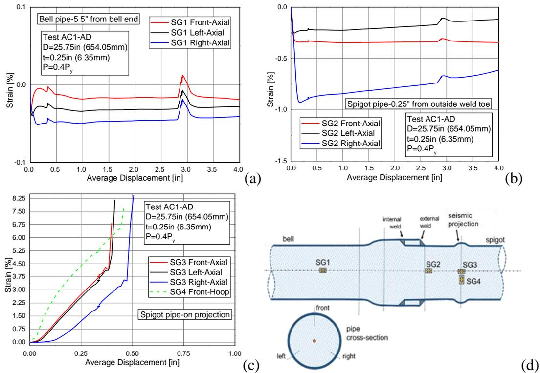
Figure 11. Strains with respect to applied displacements for axially compressed specimen AC1-AD-SR.
