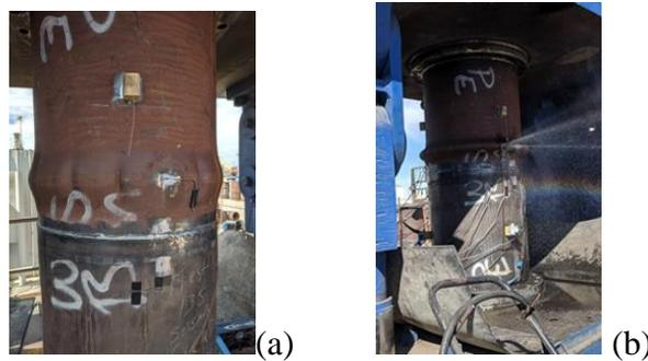
**Figure 13. (a) Deformed shape of axially-loaded AC5-BD-SR specimen; (b) failure of AC5-BD-SR specimen.**
