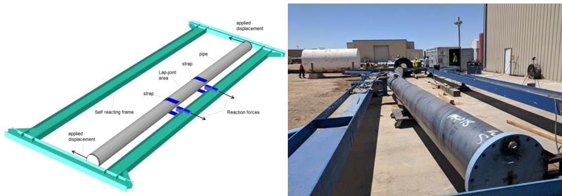
**Figure 5. Experimental setup for bending tests.**
