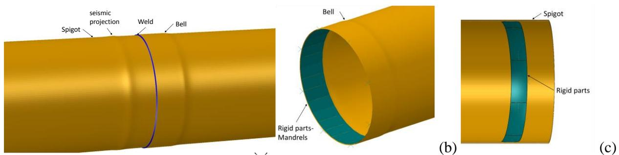
**Figure 3. Finite element model of the welded lap joint; geometry of the double-welded area of the joint.**
