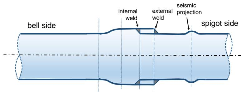
**Figure 2. Lap welded joint equipped with the artificial “seismic projection”; ALTAS SR-joint concept (not to scale).**
