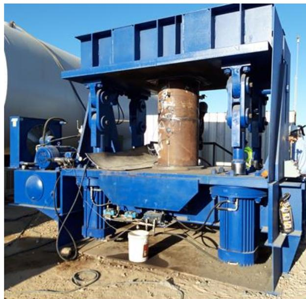
**Figure 6. Experimental setup for axial compression tests.**
