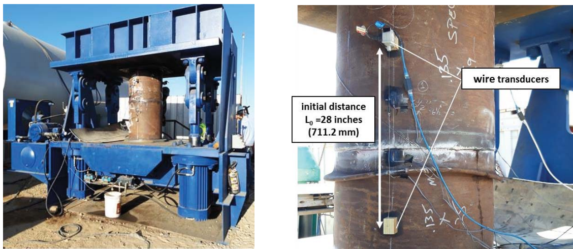
Figure 2. (a) Experimental setup for axial experiments; (b) wire transducers for the measurement of the normalized deformation of the joint \Delta L/L_0 (shortening or elongation).
