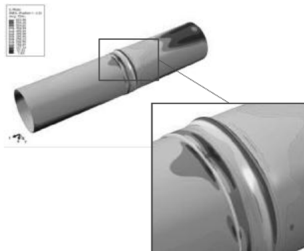
Figure 15. Deformed shape of double-welded thick pipe subjected to bending moment with zero internal pressure.
