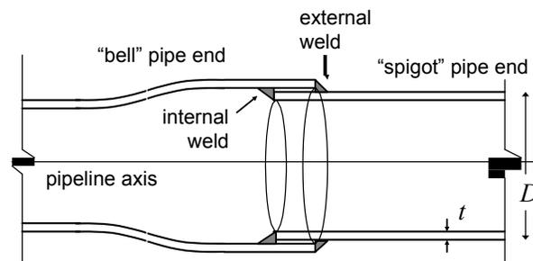
**Figure 1. Configuration of a double-welded lap pipe joint.**
