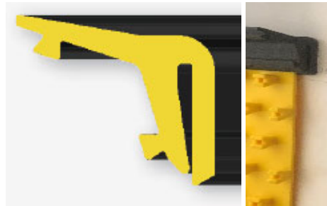
Figure 2: Liner Clip Cross Section & Image
