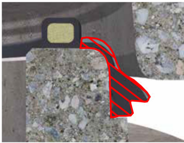
Figure 6: Section of SDV Gasket Removed
