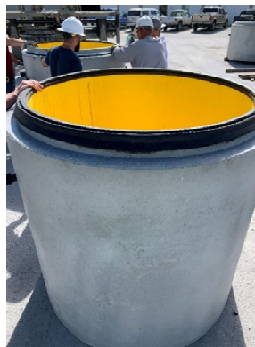
Figure 4: Manhole Base with SDV Joint Configuration
