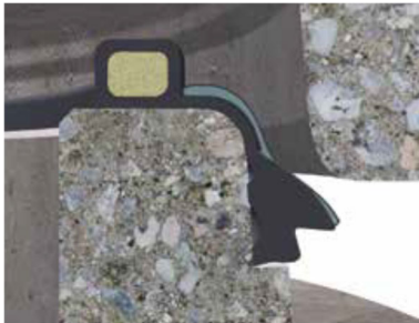
Figure 1: DS SDVseal Cross Section
