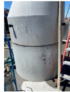
Figure 7: Quartz Sand Filled Load Transfer Hose Secondary Hydrostatic Test Manhole Stack
