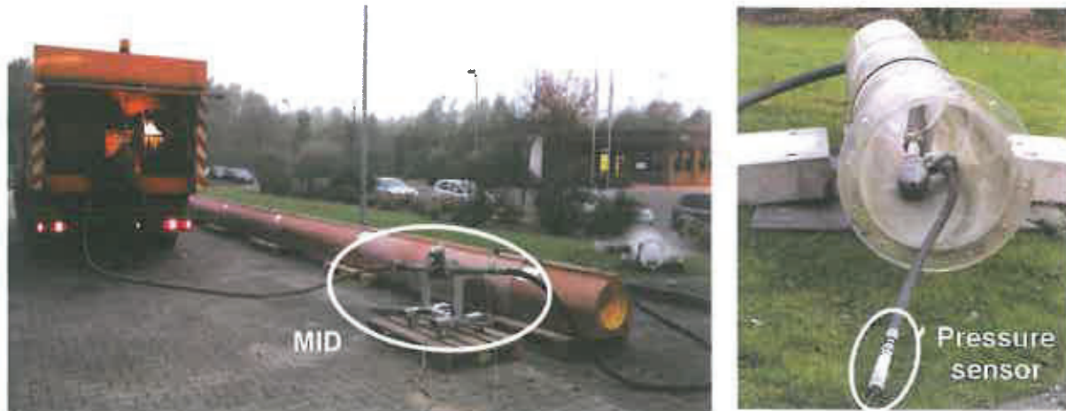
Figure 11: MID and pressure sensor for monitoring of the test parameters
