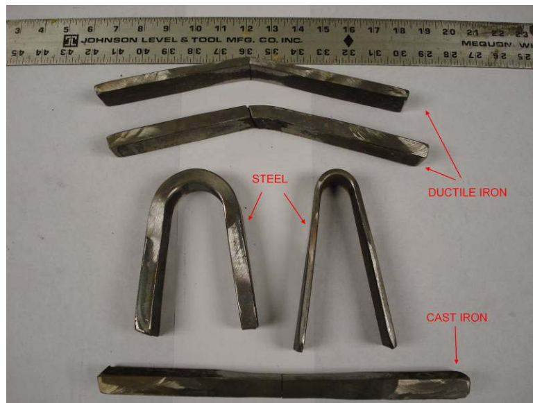
Figure 7: Bend Tests: DIP, Steel, and Cast Iron Pipe
