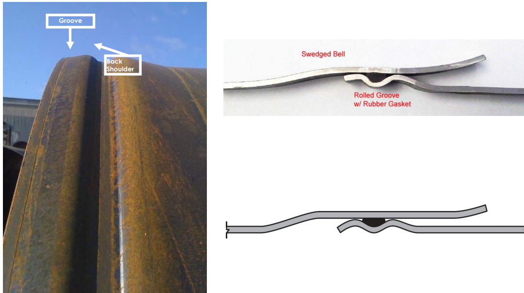
Figure 4a, b, c: Completed Rolled Groove on Spigot, Photo Cross-section of Engaged Rolled Groove Joint, Schematic of Rolled Groove Joint
