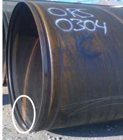
Figure 5: Grinding Flush of Spiral Weld Seam in Joint Configuration
