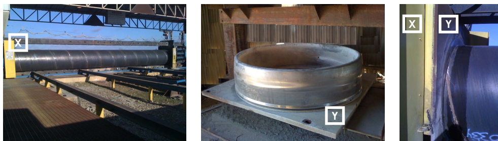
Figure 3a, b, c: Hydrotester, Hardened Bell Plug Die, Swedged Bell Forming During Hydrotesting
