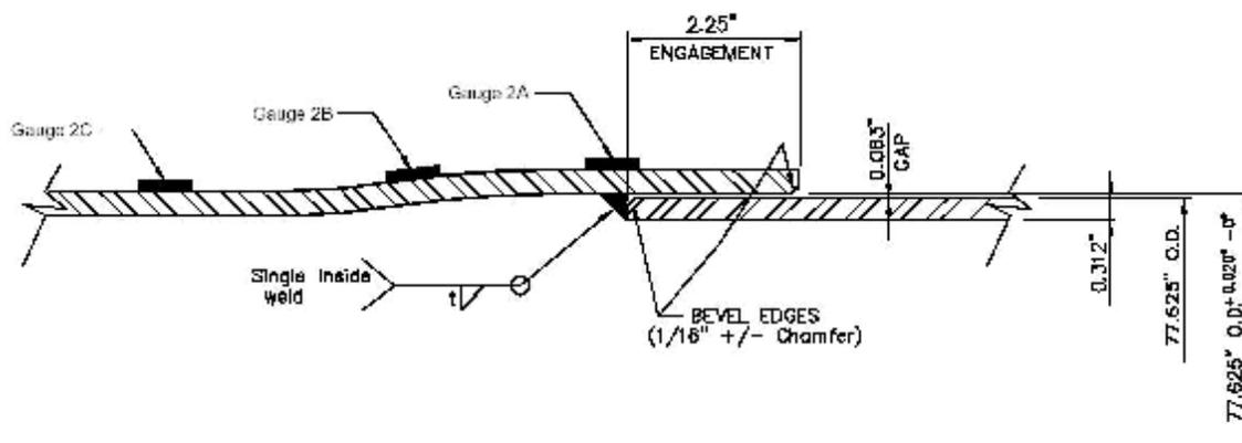
**WB X WS SINGLE WELD JOINT DETAIL**
