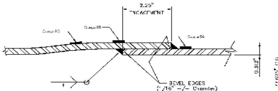
**WB X WS DOUBLE WELD JOINT DETAIL**
