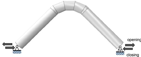
**Figure 11.** Loading pattern for elastic-plastic analysis of mitered elbows; opening and closing forces.
