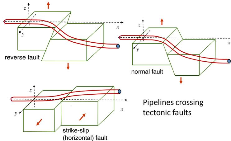
**Figure 2:** Schematic representation of pipeline configuration crossing tectonic faults.
