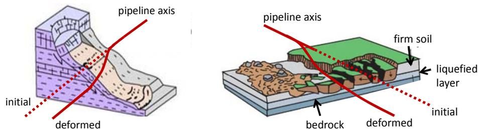
**Figure 4:** Schematic representation of pipeline configuration in the boundary of landslide (left) and liquefaction-induced lateral spreading (right) [source: USGS; <http://pubs.usgs.gov/>].
