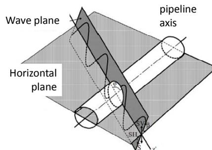
**Figure 1:** Shear wave analysis, oriented randomly with respect to the pipeline.
