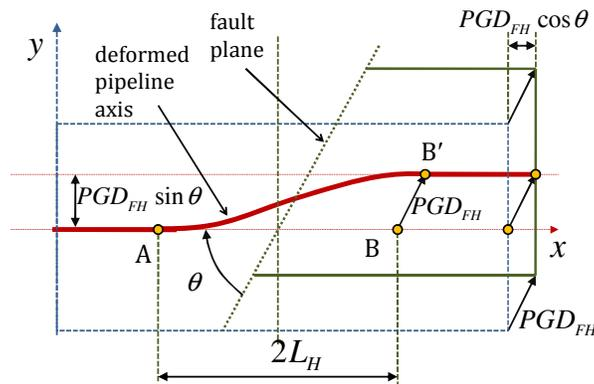
**Figure 3:** Pipeline deformation crossing a horizontal fault at angle  $\theta$ .
