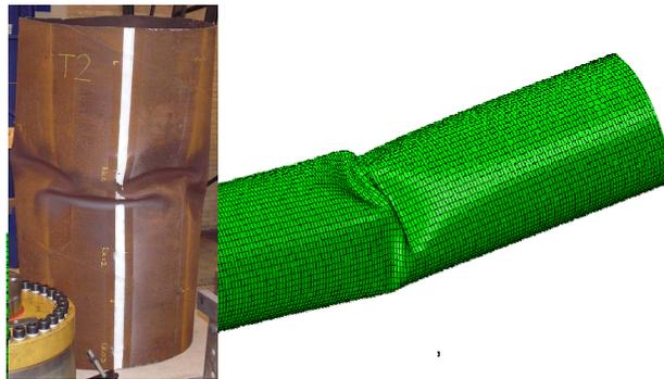
**Figure 6:** Local buckling of spiral welded pipe with  $D/t = 119$  due to excessive pipe wall compression, subjected to longitudinal bending [Vasilikis *et al.*, 2014].
