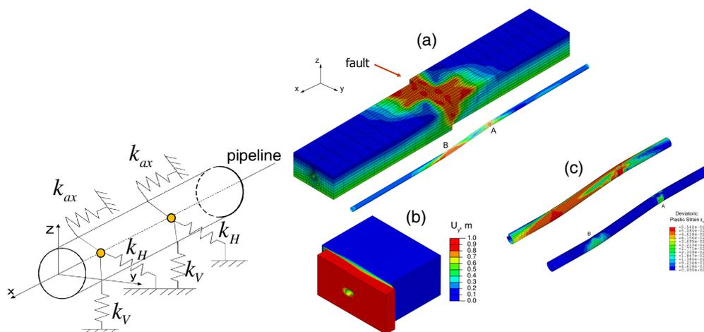
**Figure 5:** Level 1 of pipeline modelling; pipe (beam-type) finite elements and soil springs attached to pipeline nodes in the three principal directions (left); Level 2 of pipeline modelling; shell elements and solid elements (right) [Vazouras *et al.*, 2010].
