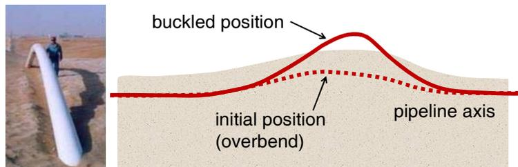
**Figure 7:** Beam buckling of buried pipeline due to excessive axial loading.
