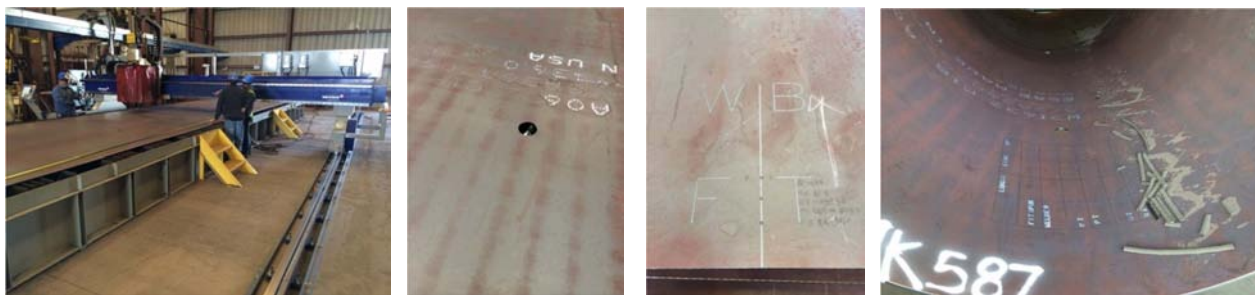
Figures 4a, b, c, d: Burn Table, Hole Cut for Grout Coupling, Orientation Etch, Grid Etched for Technical Information on Each Reliner Section
