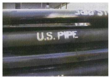
Figure 4. Ductile Iron Pipe with polyurethane coating (Szeliga/Lieu, 2002)
