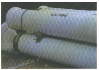
Figure 5. Tape-coated Ductile Iron Pipe (Szeliga/Lieu, 2002)
