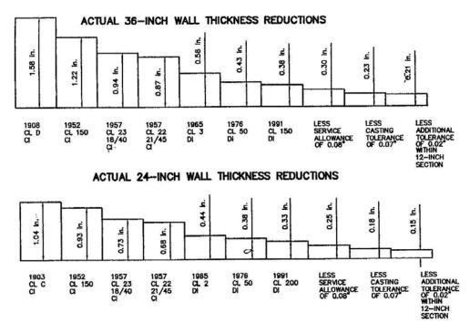
**Figure 1.** Actual Size of American Water Works Association (AWWA) Specification Thickness Reductions for 36- and 24-inch Diameter Cast and Ductile Iron Pipe 1908 to present (150 psi Operating Pressure) (Spickelmire, 2006)
