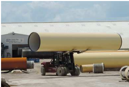
Figure 14: 108" pipe on padded forks in manufacturing facility
