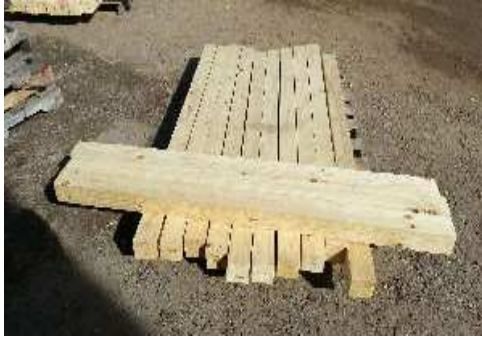
Figure 5: A pallet of stulls ready for use
