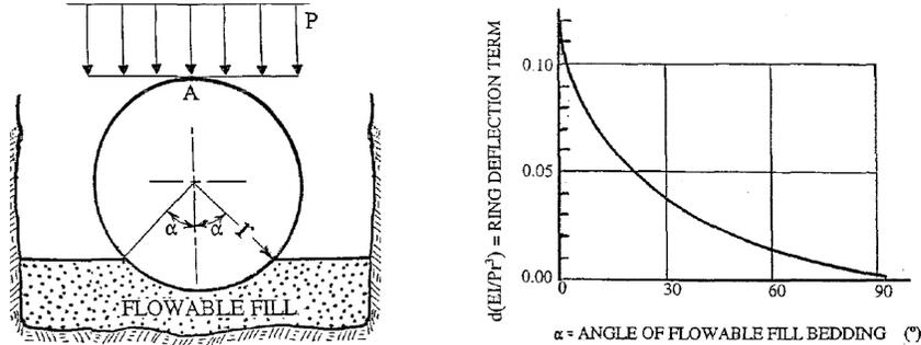
**Figure 5a, b: Flowable Fill Bedding, Ring Deflection-Bedding Angle Relationship (ASCE 2009)**
