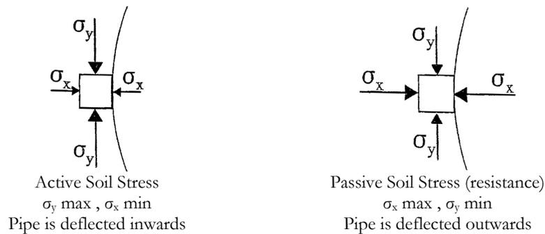
Figures 4a, b: Active and Passive Soil Stresses
