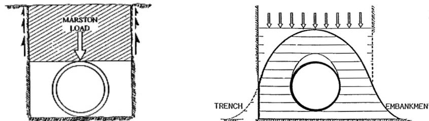
Figure 1a, b: Marston Load (ASCE 2009), and Soil Arching (Watkins 2001)
