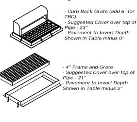
Manholes and Combo Boxes with Ring and Cover Suggested Cover over top of Pipe - 23 Depth to Invert Shown in Table.
