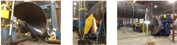
Figures 5a, b, c: Submerged Arc Welding, Plasma Cutter, Forming of Weld Bells
