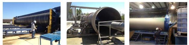
Figures 6a, b, c: Hydrostatic Testing, Cement Mortar Lining, Polyurethane Coating
