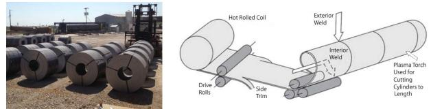
Figures 4a, b: Steel Coils, Schematic of Spirally Welded Steel Cylinder Manufacture
