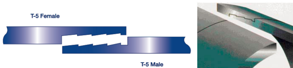
Figures 6a, b: Cross-Sections of the Permalok T5 Joint
