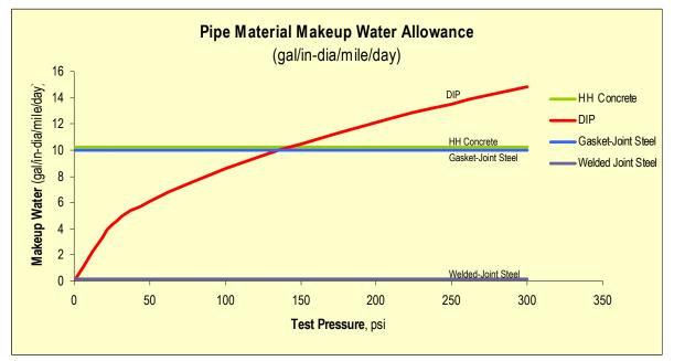
Note: Since the term "no significant leakage" for welded-joint steel pipe could be interpreted differently by contractors than by project owners, the next revision of AWWA C604 (currently being reviewed at the Committee level) will recommend a test allowance of 10 gal/in-dia/mile/day for steel pipe with welded joints, gasket-sealed joints, or mechanical couplings.
