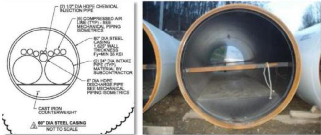
**Figure 7. Cast Iron Ingots for Buoyancy**
