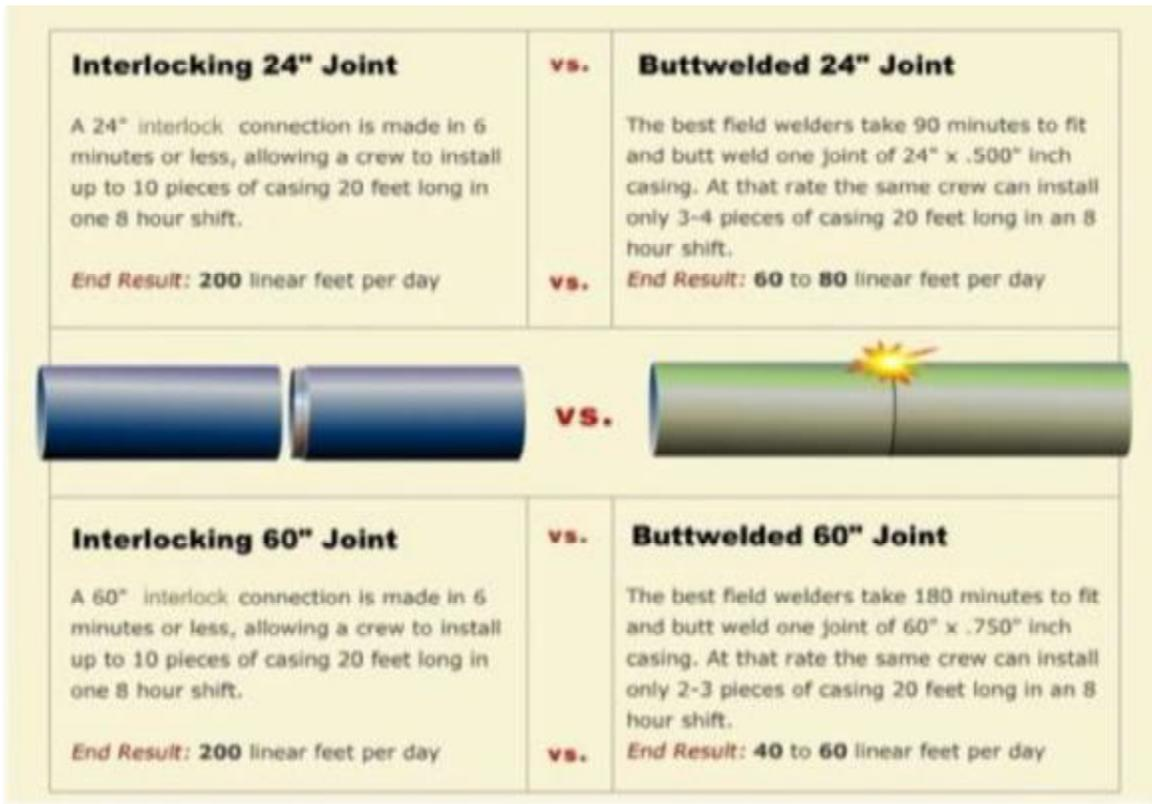
Figure 5. Interlocking Joint vs Welded Joint
