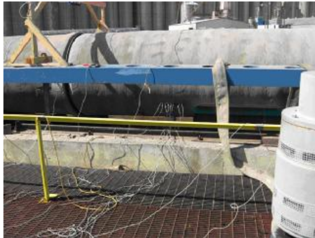
Figure 9: Strain Measurement Instrumentation Attached to Prototype
