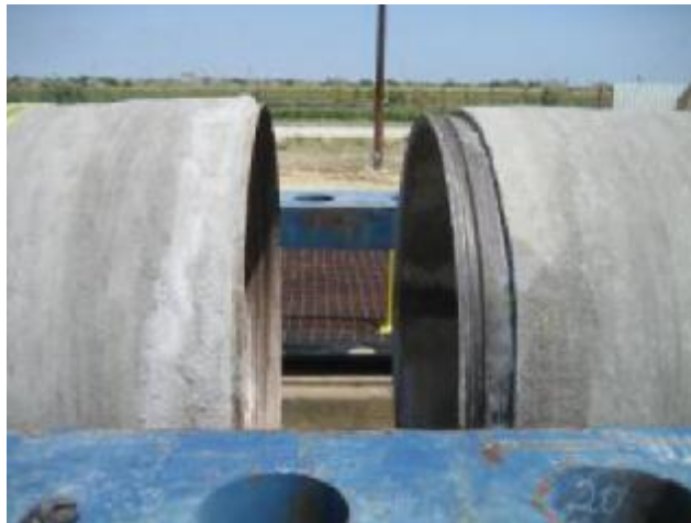
Figure 8: Swedged Bell and Spigot w/ Rolled Groove Prior to Assembly
