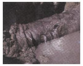
5-year old ductile-iron pipe in polyethylene encasement
