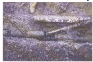
A section of failed polywrapped pipe being removed. Failure occurred from external corrosion at breaks in the wrap.
