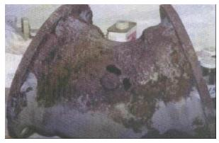
DI fitting after 15 year of service, showing widespread corrosion penetrations typical of the entire pipeline. No corrosion protection was provided for this line. The soil sample from this location scored zero on the 10-point scale, indicating essentially noncorrosive conditions.
