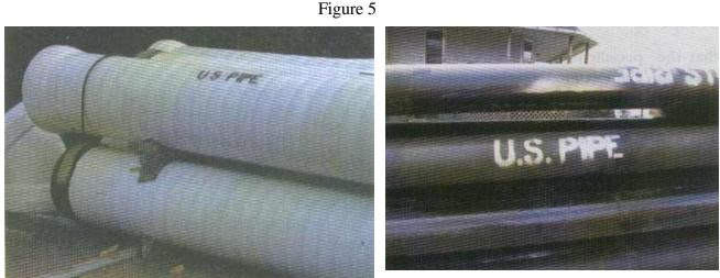
Tape-coated ductile iron pipe.
