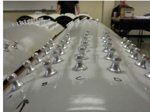
Figure 2(b). Separated, coated sections of pipe with dollies prior to adhesion testing.
