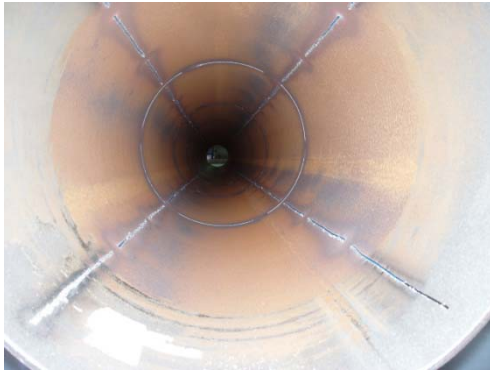
Figure 2(a). Internal view of precut pipe (1.22 m) after coating, but before final separation of the sections.
