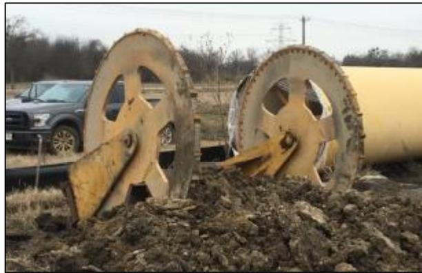
**Figure 5: Wheel Compactor for Granular Embedment**
