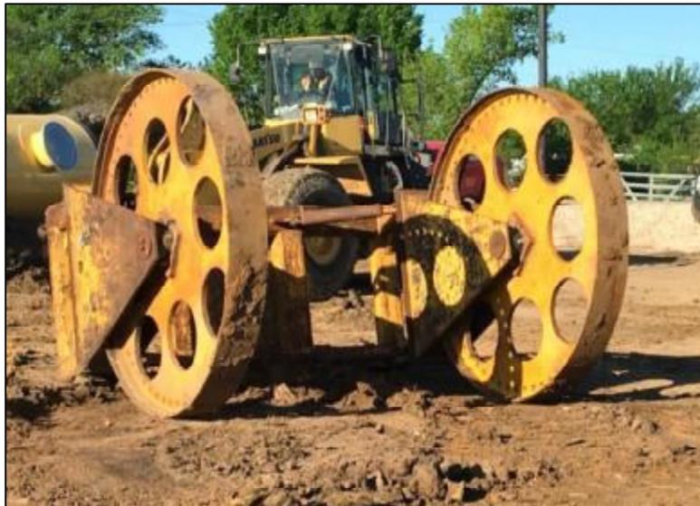
**Figure 7: Wheel Compactor for CSS Embedment**
