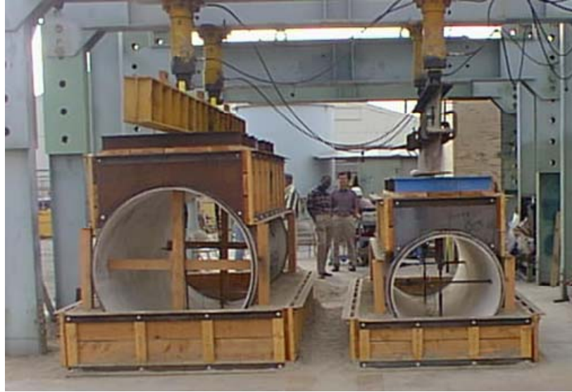
Figure 2. Set up for Sand-Bearing Load/ Deflection Tests
